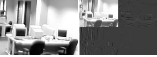
Figure 3: An image patch and its Haar decomposition. The four bands in the image on the right correspond to B^l (top-left), B^v (top-right), B^h (bottom-left) and B^d (bottom-right)
