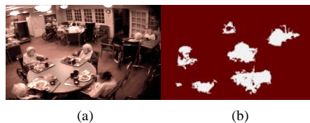
Fig. 2. Finding individual person. (a) A frame of the video. (b) The individual person regions obtained using our method (duration is 2 minutes).
