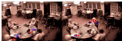
Fig. 1. Automatically estimated moving regions and motion vectors. The red arrows are computed motion vectors; the blue masks indicate segmented moving regions.
