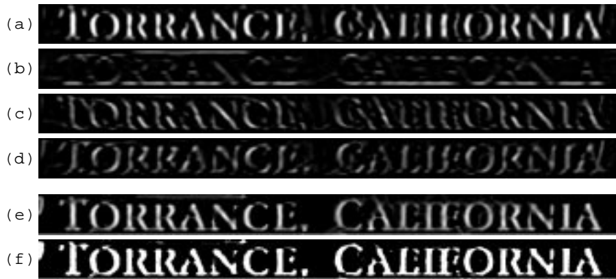
Figure 9: Result of character extraction filter. (a) Vertical. (b) Horizontal. (c) Left diagonal. (d) Right diagonal. (e) Integration of four filters (f) Binary image.
