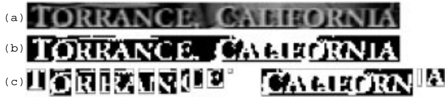
Figure 7: (a) Original image ( 204 \times 14 pixels). (b) Binary image. (c) Character extraction using a conventional technique.
